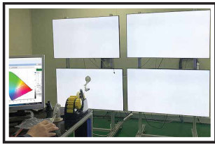
Factory tuning color calibration of white balance
